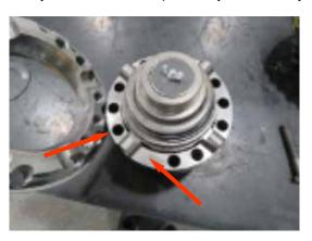
5. Lay the diff assembly on its side to install the new top plate bolts. This will keep the top plate in place until you get the bolts started by hand.
