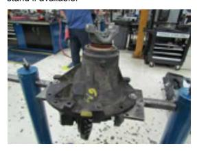
Before we start to disassemble the carrier, we need to measure the ring gear backlash. We will be resetting the backlash to this setting when we reassemble the carrier.
