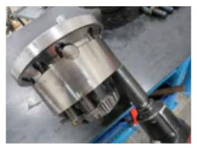
7. We can now install the two new alignment dowels. Use a press or hammer to fully seat them in the top plate.
