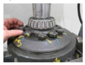
11. Slowly press the gear in place. Having the ring gear bolts installed will guide the ring gear, keeping it from misaligning during the press.
