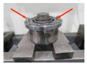
10. The ring gear can now be lowered on to the diff with the dowel pins in alignment. Before we press the gear to the diff case, we want to start all the ring gear bolts by hand, engaging a couple of threads.
