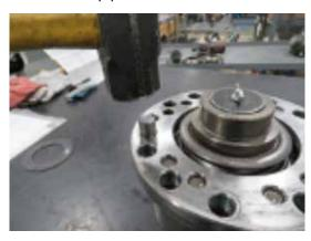
Install the thick thrust washer to the NoSPIN. Oil both sides.
