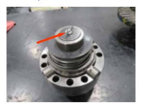
**Important:** Do not remove the wing nuts holding the NoSPIN together. It must be installed into the diff case fully compressed.
