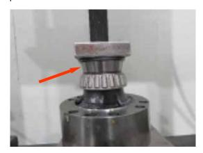
Install the inner thrust washer. Apply oil to each side.
