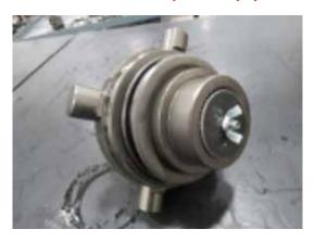
4. The differential top plate can now be installed over the NoSPIN. Remember the bolt holes are not symmetrical, so the plate only fits one way.
