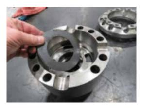
3. We can now install the NoSPIN assembly. Make sure the wing nut holding the NoSPIN together is facing up; this will make it easier to remove later in the procedure.
